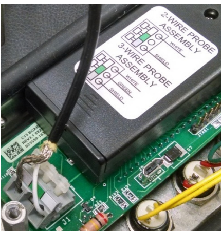
Figure 1: Probe Assembly Lead Attachment
