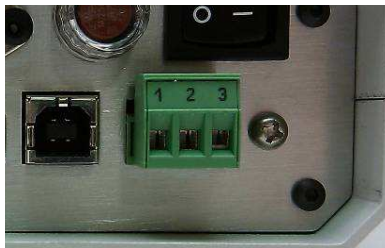
Figure 1: Relay screw-terminal header
